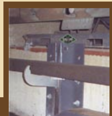
Positive Contact Hook captures and holds all legal ICC Bars.
